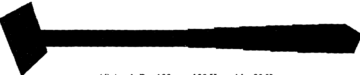
Figure 6.7: Optimal solution of the cantilever beam with various design parameters
